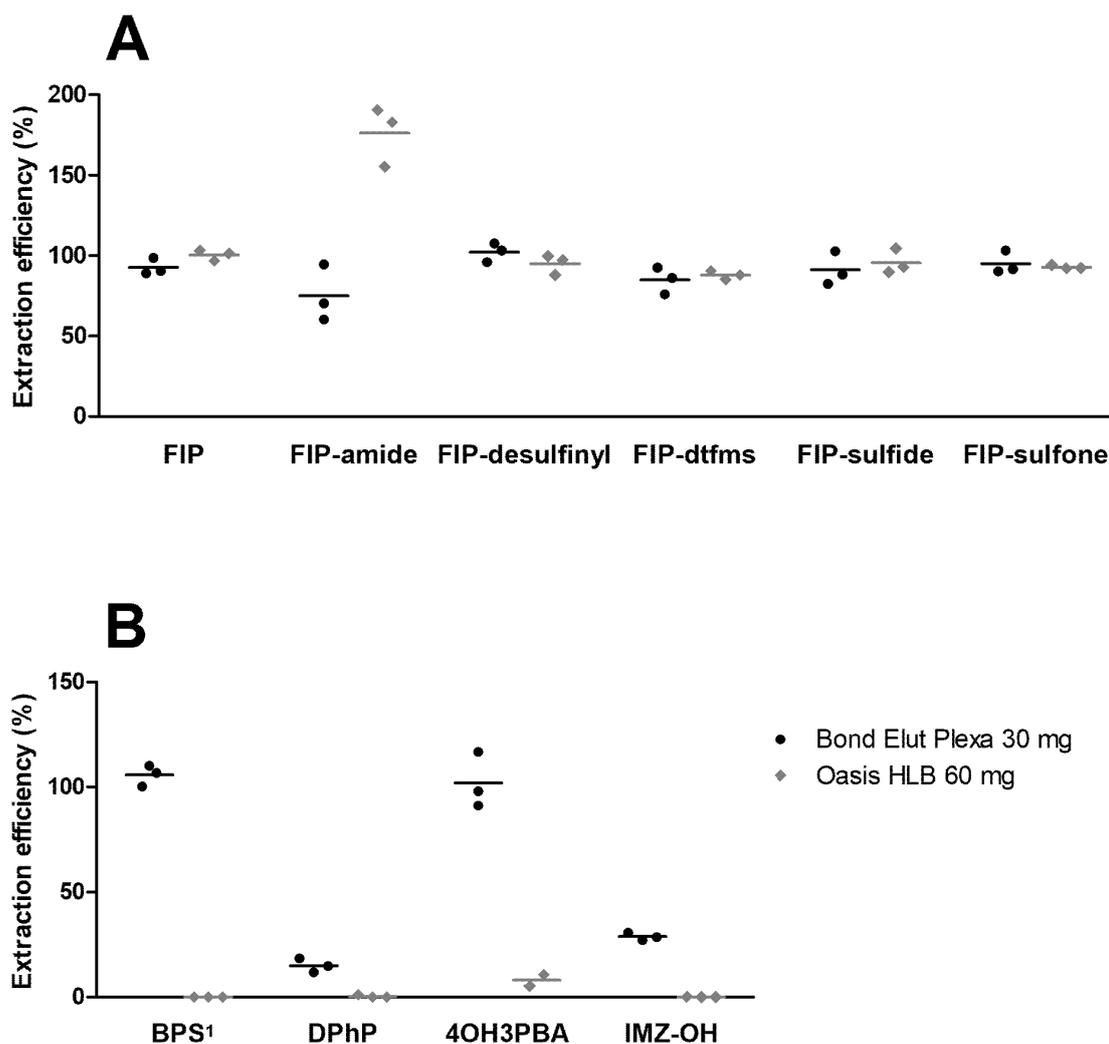
Figure 4.2 Comparison of extraction efficiencies for fiproles (A) and selected other analytes (B) obtained using Bond Elut Plexa 30 mg and Oasis HLB 60 mg.
