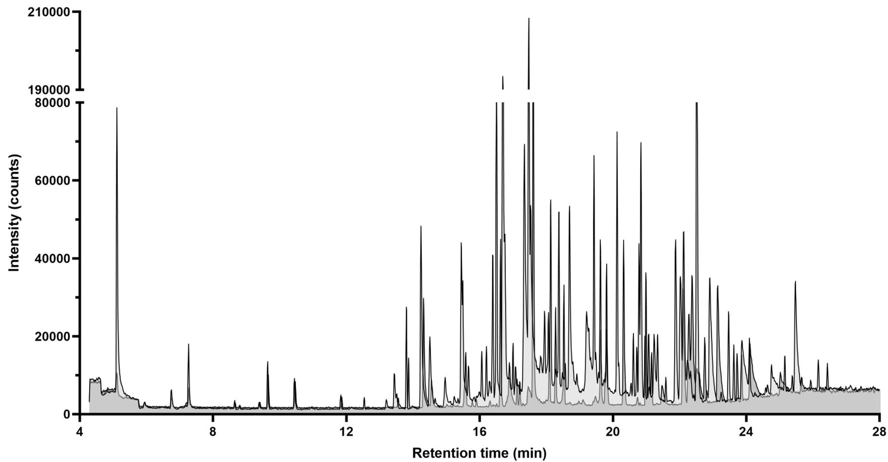
Figure 4.8 Comparison of TIC chromatogram of sample without cleanup (black line, light grey fill) and sample after freezing-out and LLE with n-hexane (grey line, dark grey fill).
