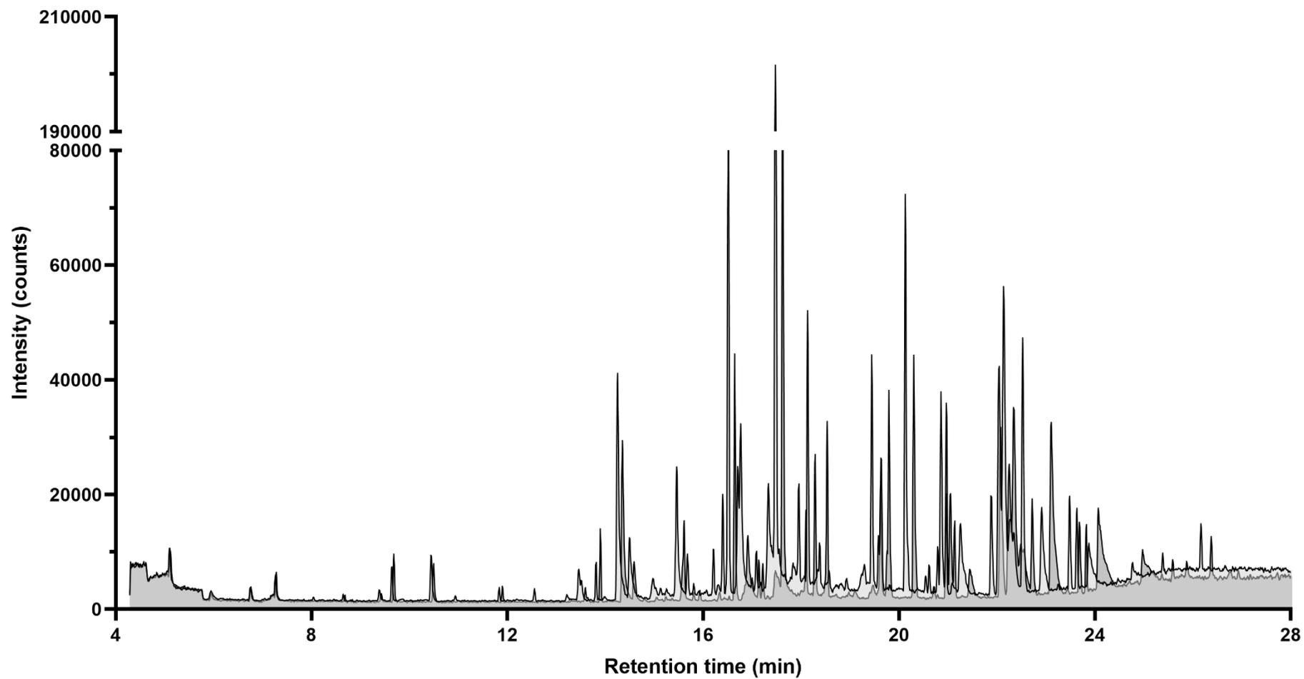
Figure 4.9 Comparison of TIC chromatogram of sample after freezing-out (black line, light grey fill) and sample cleaned up using freezing-out and LLE with n-hexane (grey line, dark grey fill).
