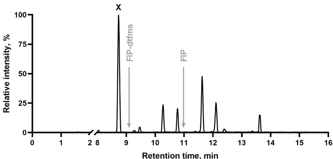
Figure 4.4 Total ion chromatogram of FIP-OH standard in negative ionization. Peak that was subject to further investigation is marked by "X". Retention times for FIP-dtfms and FIP are indicated by grey arrows.
