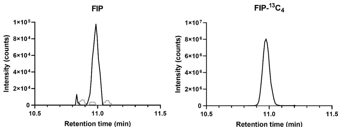
Figure 4.6 Signal of FIP and FIP- $^{13}\text{C}_4$  in spiked (black line) and unspiked (grey line) samples. In the spiked samples, the signals correspond to concentrations equal to 1  $\mu\text{g}/\text{mL}$  and 200  $\mu\text{g}/\text{mL}$  for FIP and FIP- $^{13}\text{C}_4$ , respectively. Only the quantitative transitions are shown for clarity.
