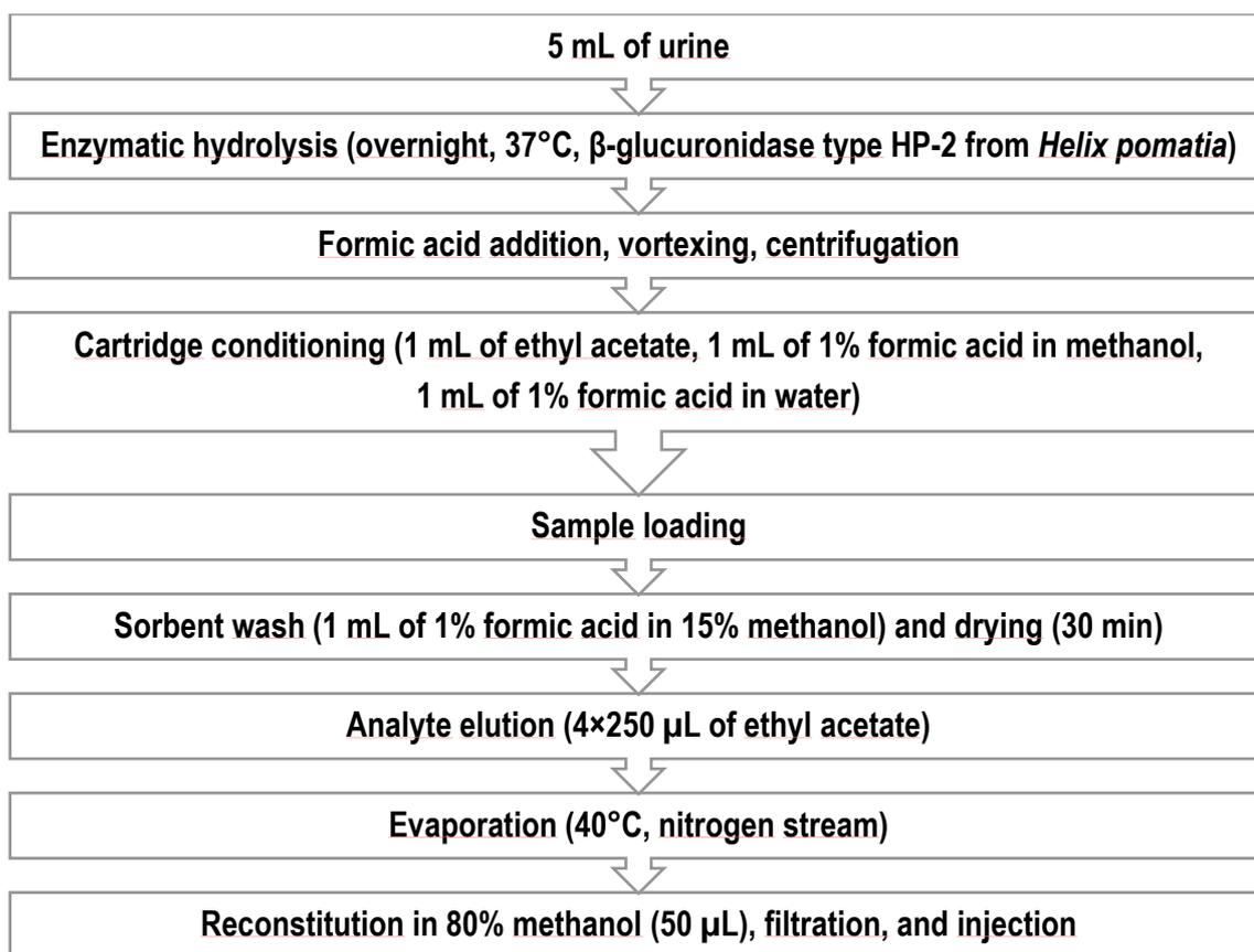
Figure 3.1 Workflow of the final sample preparation procedure for urine samples.
