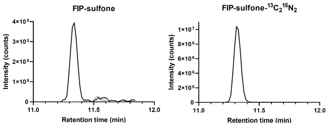
Figure 4.12 Signal of FIP-sulfone and FIP-sulfone- $^{13}\text{C}_2^{15}\text{N}_2$  in spiked (black line) and unspiked (grey line) samples of SWBs. In the spiked samples, the signals correspond to concentrations equal to 0.1 ng/g and 9.6 ng/g for FIP-sulfone and FIP-sulfone- $^{13}\text{C}_2^{15}\text{N}_2$ , respectively. Only the quantitative transitions are shown for clarity.
