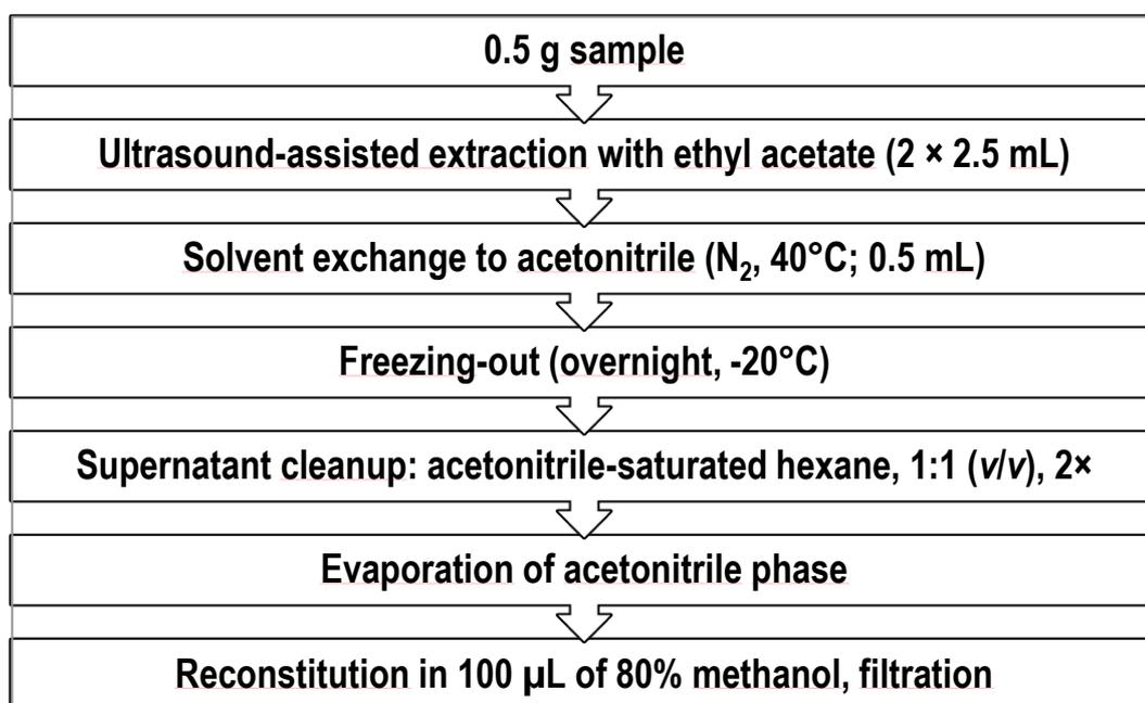
Figure 3.2 Workflow of final sample preparation procedure for silicone wristbands.
