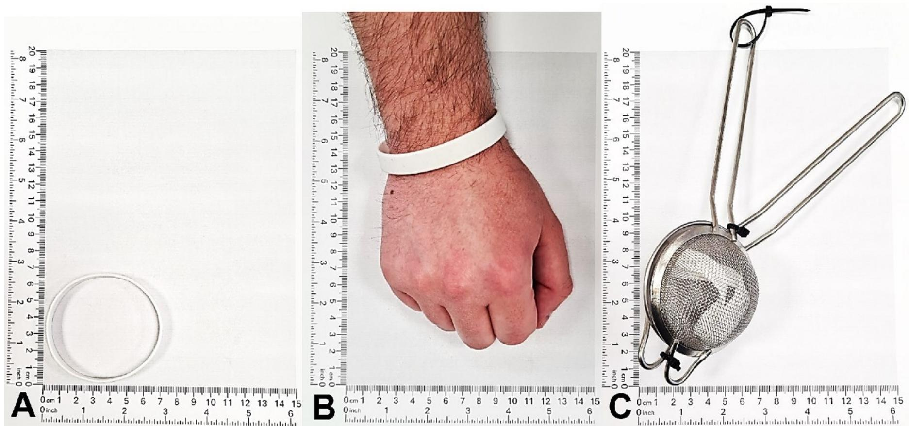
Figure 1.4 A silicone wristband (A), a silicone wristband worn during an exposure assessment study (B), and a silicone wristband in a stainless steel housing to be used as a stationary sampler (C).
