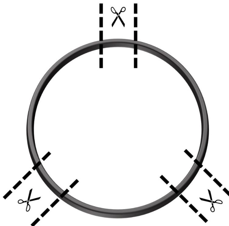
*Figure 3.3 Sampling method for homogeneity test of silicone wristbands.*
