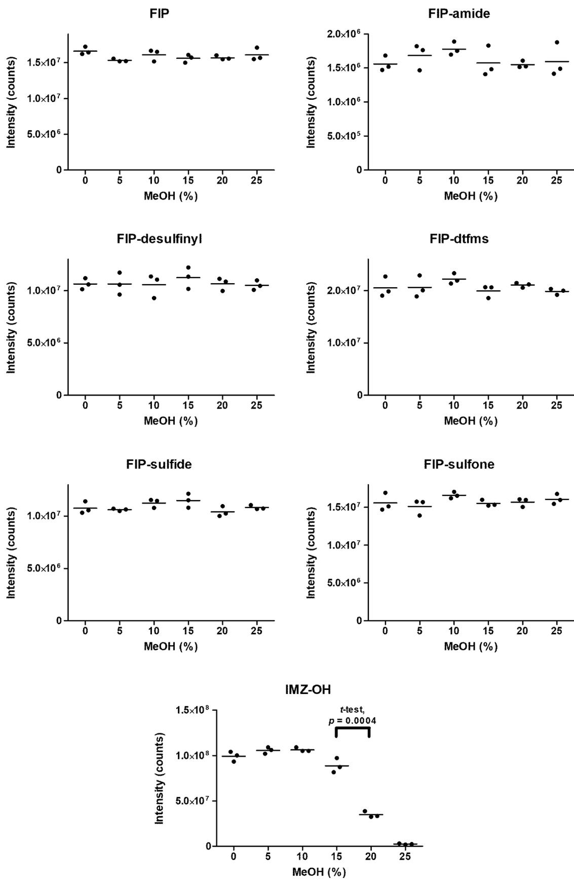
Figure 4.3 Effect of wash solution composition used during SPE procedure on analytical signal of selected compounds.
