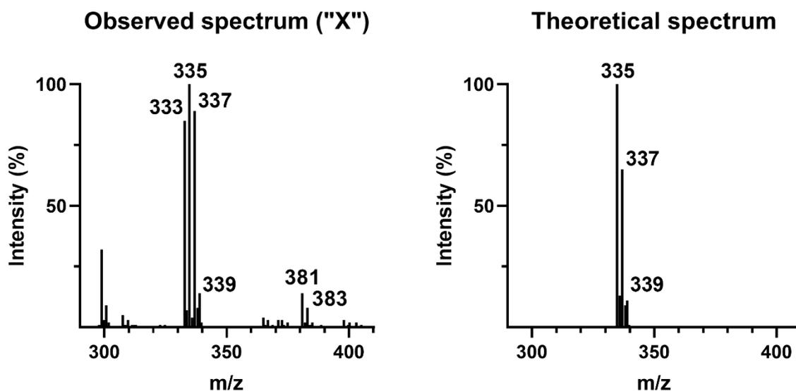
Figure 4.5 Spectrum of peak "X" (left) and theoretical spectrum expected for FIP-OH (right).
