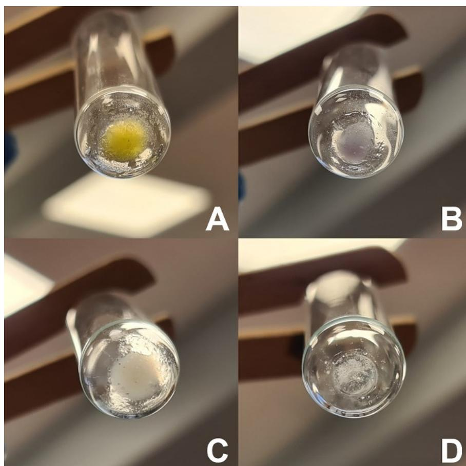
Figure 4.7 Dry residue after evaporation of ethyl acetate extract of used (A-C) and unused (D) wristbands. Note the oily residue in used samplers. All wristbands were in the same color (white).
