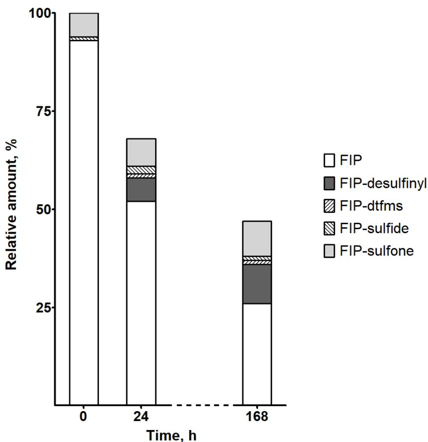
Figure 4.11 Relative amounts of FIPs during simulation study of outdoor stability of FIP spiked on SWBs. All amounts relative to molar sum of FIPs at  $t = 0h$ . FIP-amide was omitted (not detected).
