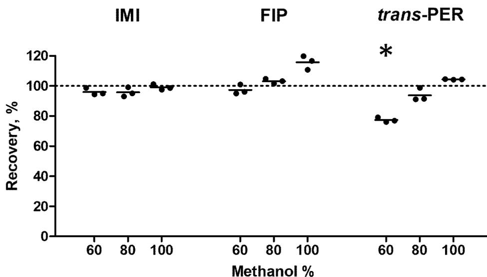
Figure 4.1 Analyte loss due to filtration. A dashed line at 100% recovery was added for reference. An asterisk denotes a statistically significant difference ( $p < 0.05$ ).
